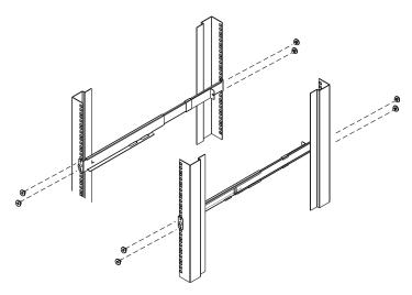
3. Slide the switch onto the support flanges. Use the screws supplied with this package to loosely attach the front of the switch to the front of the rack (only tighten the screws part way).
